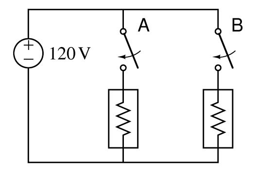
You are assigned the task of creating a light fixture for use in a home. The resistors represent the filaments in the light bulb. The light bulb is supposed to be a three-way bulb with light of 50 Watts, 100 Watts, and 150Watts. When only switch A is closed, the bulb should consume 50Watts, 100 Watts when only switch B is close, and 150 Watts when both are closed. Design the resister values to match this case.
