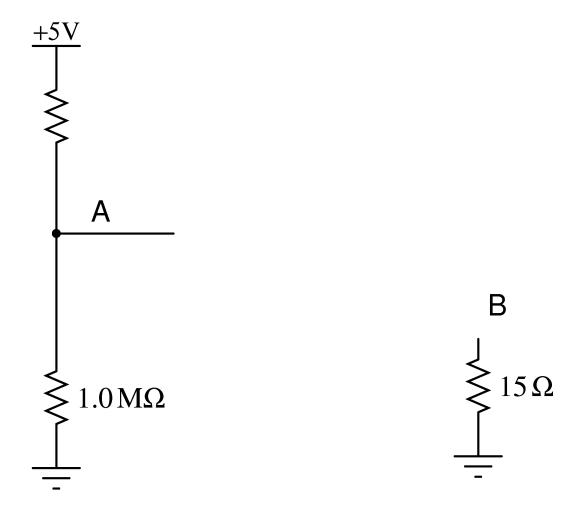
The above diagram shows some of the parts in a design for a nightlight. When the room is dark enough, the voltage at A will drop to 0.5 volts. At this point, voltage should be applied to B, which will light the small lamp to provide a nightlight. The lamp's resistance is  $15\Omega$ , and is designed to operate at 15W. Design a circuit that will deliver 15W of power to B whenever the voltage at A is below 0.5 volts. The additional components must not use more than 2mW.
