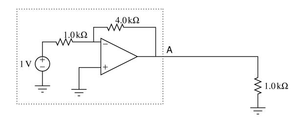
The above circuit is a representation of an amplifier that was designed to amplify the signal from the 1V source by a factor of 4 for the  $1k\Omega$  load. The amplifiers come with two in each package. The problem is when the circuit was placed in the board; the Op Amp was supplying too much current at its output and no longer operating in it linear range. The amp can only deliver 4mA within its linear range. Can you rewire the circuit to amplify without drawing too much current?
