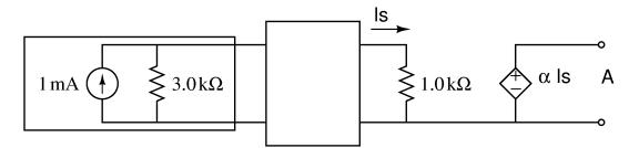
The above is a partial circuit design for an amplifier. The output at A is rated to be 3V when the input is 1mA.  $\alpha$  is equal to 5V/mA. Design an interface circuit that will meet these conditions.
