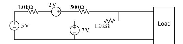
The above circuit represents the series of patches made to a power supply over time. As the load changes, so did the power supply requirements. Before this turns into even more of a mess, your boss asked you to come up with a simpler design that will accomplish the same job. The simpler design must use fewer components and work exactly the same no matter what the load is. Design an equivalent circuit that does the job.
