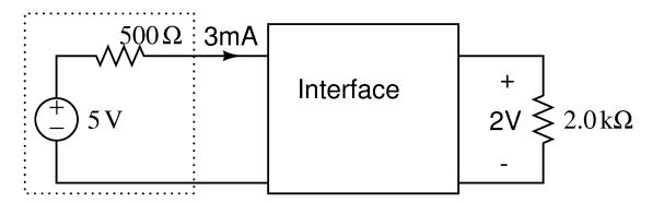
In the same car CD player design, the reading laser needs to be supplied with 2 Volts, which has a resistance of  $2k\Omega$ . This can easily be solved by a voltage divider except that the voltage source is not stable unless 3 Amp are pulled from it. Design a combination voltage and current divider that will pull 3 Amps from the voltage source and still provide 2 Volts to the laser.
